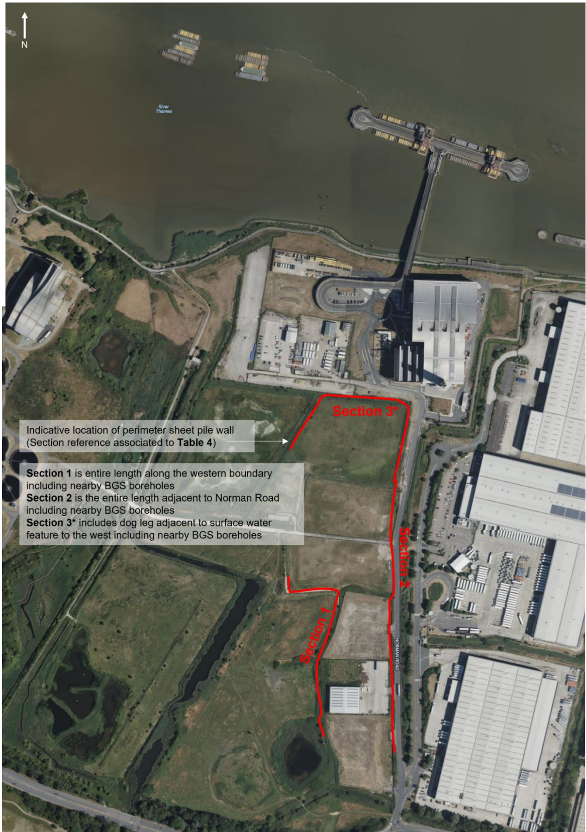
Figure 3-1: Indicative Perimeter Sheet Pile Wall and Section References for Groundwater Impact Assessment (see Table 3-1)
